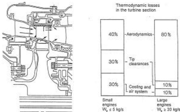
Fig. 7: Thermodynamic losses in the turbine module
