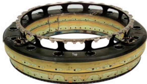
Fig. 5: Thermo colours pattern after the rig test
