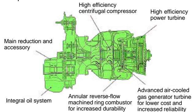
Fig. 2: Engine architecture
