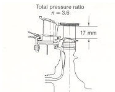
Fig. 6 Single stage transonic high pressure turbine
