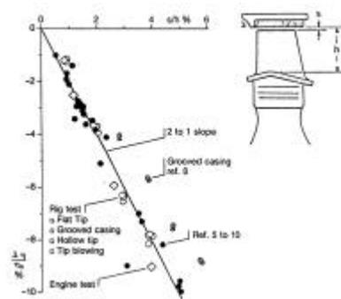
Fig. 8 Influence of tip clearance variations on stage efficiency
