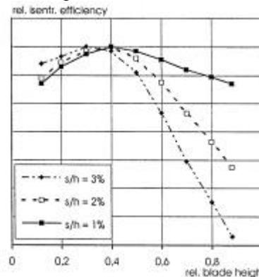
Fig. 9: Influence of tip clearance variation on the radial efficiency distribution
